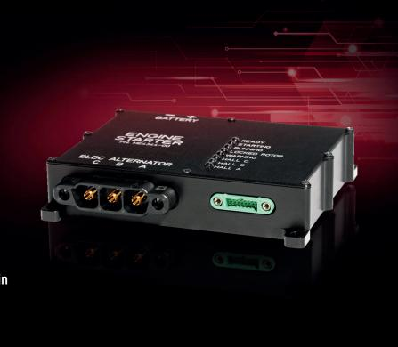
The engine starter drives the BLDC generator as a motor in order to start the engine. Once the engine is running the starter disconnects itself from the BLDC alternator to allow electrical power generation. A suitable BLDC alterator fitted with HALL sensors is required. Engine starting is initiated locally by push-button or remotely using CAN or RS-232 commands. In-flight restarts are possible via CAN or RS-232.
