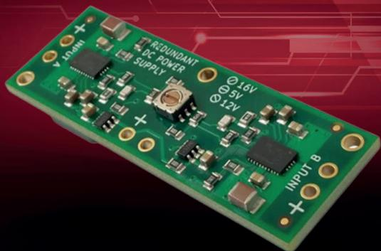
The Redundant DC Power Supply consists of two identical DC-DC switching converters and a low-loss (ideal diode) power combining stage. It is intended as a high-reliability source of power for mission critical UAVs sub-systems.
