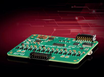
The 15S Battery Cell Monitor & Balancer is a precision instrument that ensures multi-cell batteries are maintained in an optimal state, improving system reliability and prolonging battery life.
